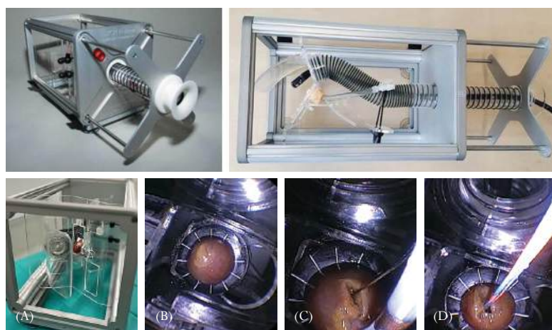
FIGURE 2 Boškoski-Costamagna ERCP Trainer with specific papilla to train on ERCP steps: biological papilla made out of chicken heart tissue (A); sphincterotomy (B); cannulation (C)
