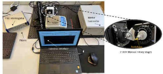
Fig. 6: Experimental setup for the data collection of the force sensor during calibration.
