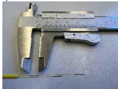
(b) The fibers are pretensioned and the FBGs are inside the nitinol tubes.
