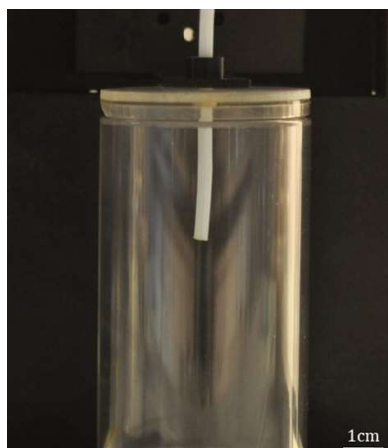
Figure 4. Setup for plume imaging in confined atmosphere. The same setup is used for imaging in ambient air with the glass container removed.
