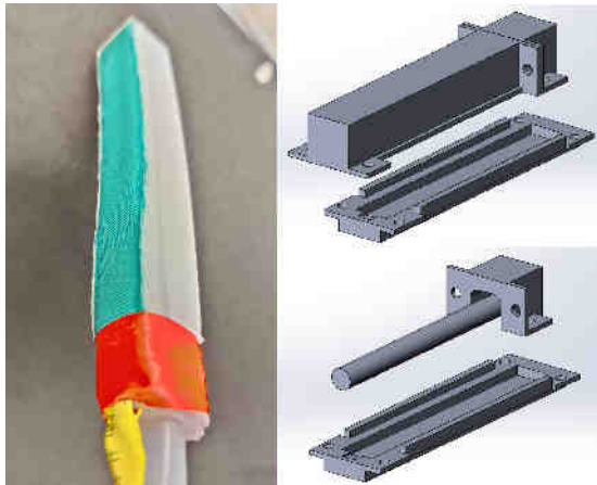
Fig. 3: Physical soft actuator (left) - CAD molds model (right)
